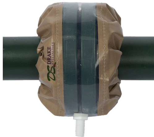
Clear PTFE flange shield: FEP window for inspection, PTFE drain nipple below.
